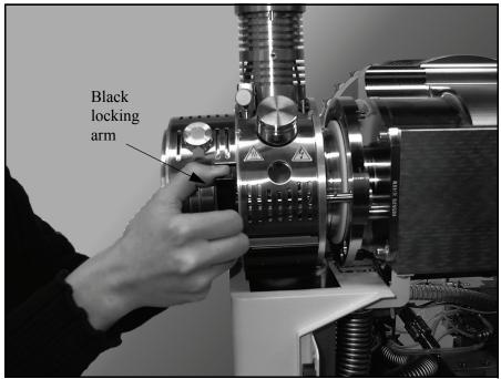
Mounting the Turbo V<sup>™</sup> source housing
