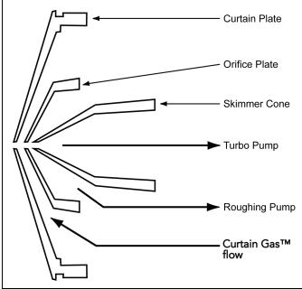
Cutaway view of the vacuum interface
