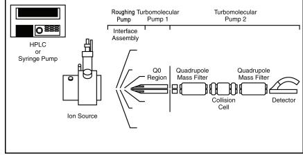
API 4000<sup>™</sup> system components with pump
