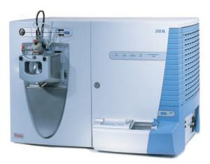
The Thermo Scientific<sup>™</sup> LTQ XL<sup>™</sup> linear ion trap mass spectrometer
