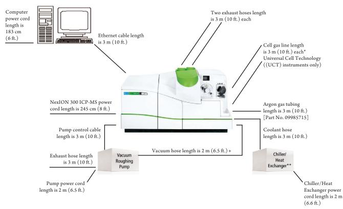
Figure 3. Location and length of connections.
