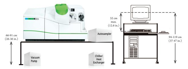
Figure 2. Recommended workstation layout.
