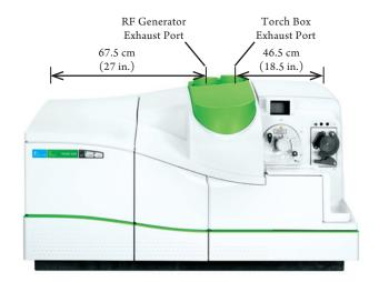
Figure 6. Location of exhaust ports.
